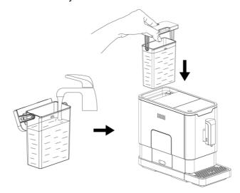
Important: Never fill the water tank with warm, hot, sparkling water or any other liquids which can damage the water tank and the machine.
