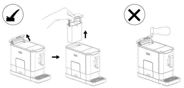
2. Rinse the water tank with fresh water and fill the tank to "MAX" level. Place it into the machine and make sure it is fully inserted.
