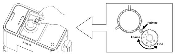
1. Only turn the knob for adjustment when grinder is in operation.
